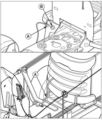
Figure 22. Rotator Motor Electrical Connection
